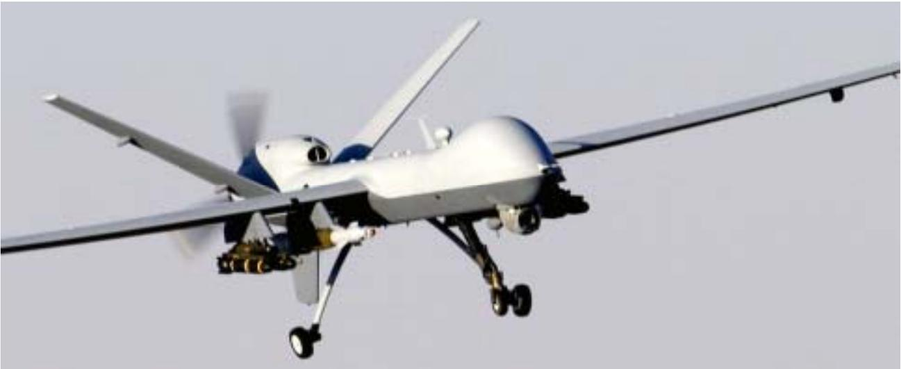
An Armed ISR UAV: General Atomics Aeronautical Systems MQ-9 Reaper. *Photo courtesy DoD.*
