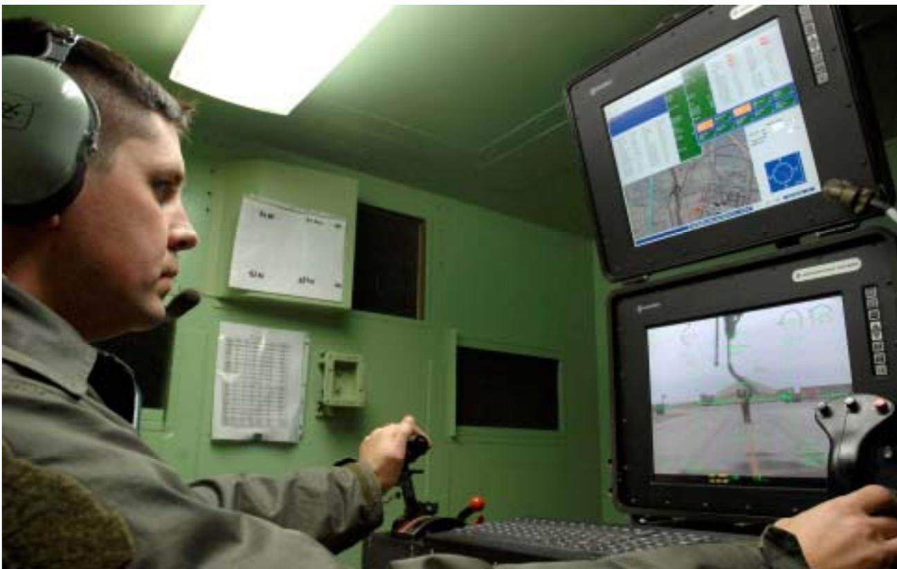
Inside the Ground Control Station of an MQ-1 Predator. Photo courtesy DoD.
