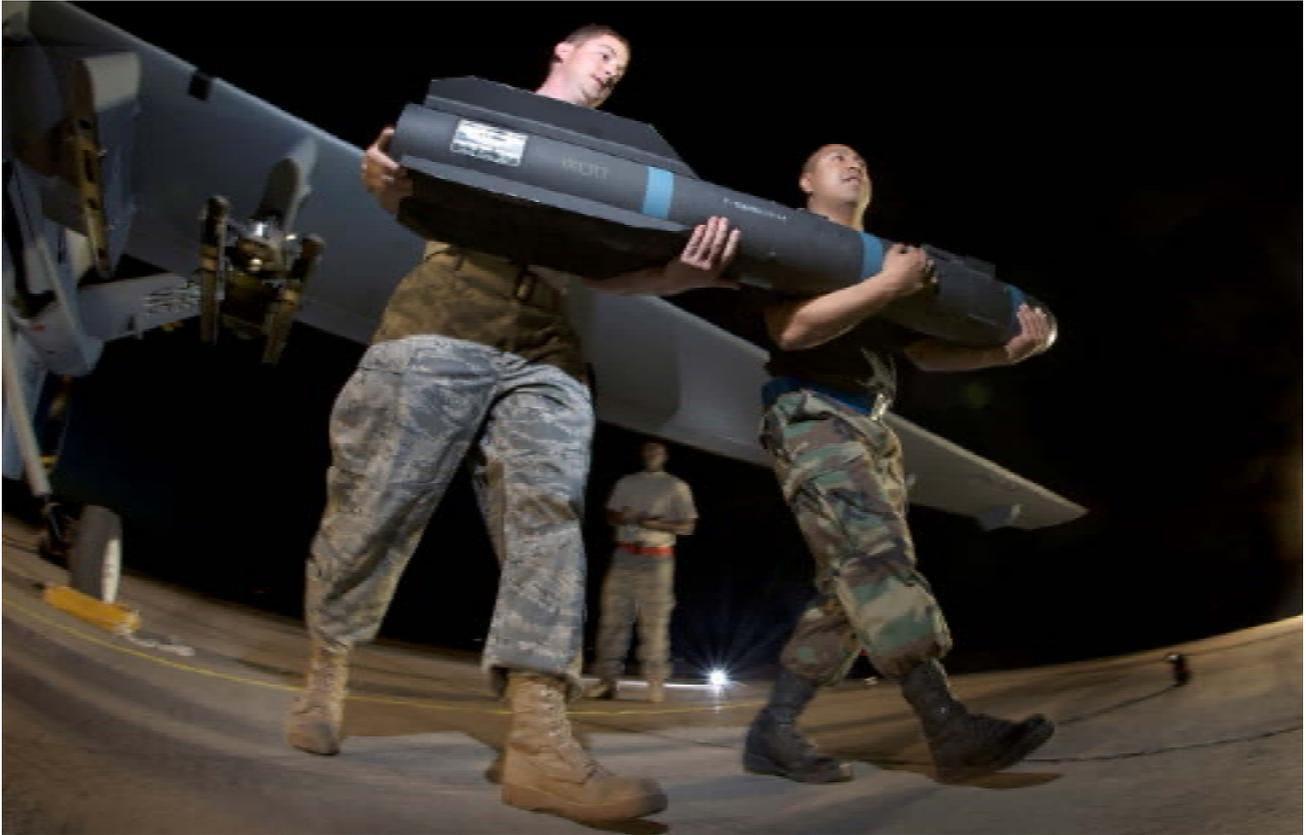
Armourers unload an AGM-114 Hellfire Missile from a MQ-9 Reaper. *Photo courtesy DoD.*
