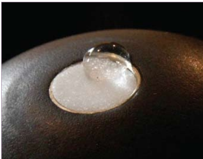
Figure 6: Droplet of water on hydrophobic-coated window. The coating prevents formation of a water film, which keeps the acoustic window sufficiently clear to avoid distortion
