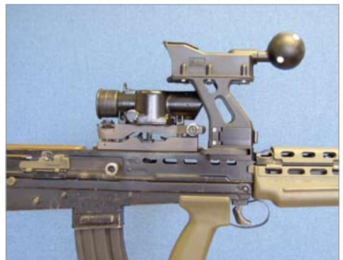
Figure 1: First generation prototype RMGL on an SA80. The gunshot detector mounts on the rifle, above or to the side of the optical sight, with a small display giving accurate localisation of the shooter, mechanically aligned with the sight. The sensor gives direct benefit to the soldier, but can also be networked to improve situation awareness at the platoon commander level and above
