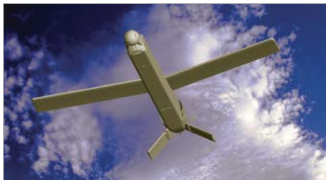
Fireshadow in flight but with the sensor rolled back for protection during transition to the area of operation [MBDA]
