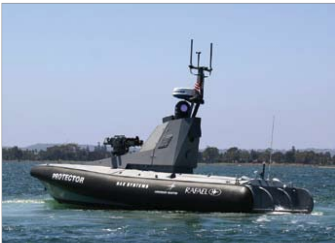
The Raphael Protector USV is equipped with a Typhoon mini-gun and Toplite Electro Optical system [BAE Systems]
