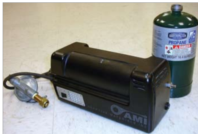
AMI-developed Solid Oxide Fuel Cell. This is a 25W system that utilises propane cylinders
