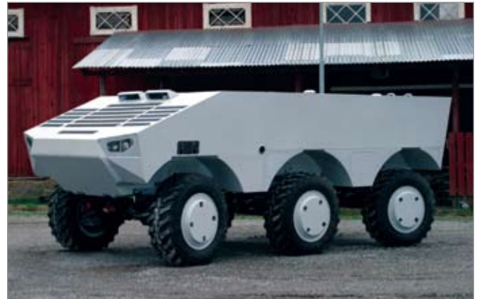
SEP is a Swedish design for an APC which pioneered in-wheel electric drive [FMV]
