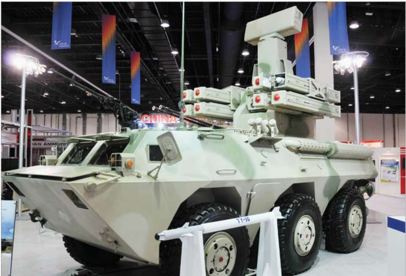
Yitian short-range air defence system on a WZ551 chassis armed with TY-90 surface-to-air missiles [Allen/Jane’s HIS Global]
