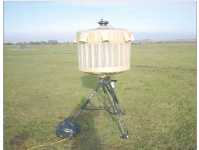
The Lightweight Counter Mortar Radar is valuable in providing vital warning of incoming indirect fire [MoD UK]
